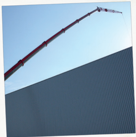
If the load and load environment are out of sight, the danger of crane accidents increases significantly.
